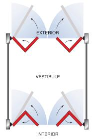
Our door panels fold in or out for the most efficient use of space at entrances or exits.
